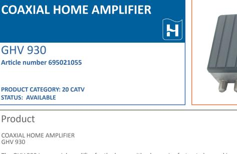
The GHV 930 is a coaxial amplifier for the home with a low noise factor, to be used in small to medium-size CATV systems in homes with more than one connection. The GHV 930 is a modular design with the option of passing on a return signal. Rotary switches and jumpers are installed on the inside to enable convenient attenuation and levelling. The return can be switched on or off, set to active or passive and the downstream can be extended to band I (in which case the return is switched off).
